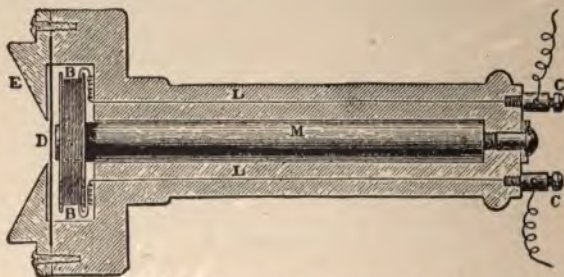
FIG. 61.—Bell single pole magnet telephone enclosed in wooden case.
